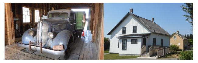
In the green Alberta Wheat Pool elevator, a 1938 Dodge truck adds to the authenticity of the elevator's operation. The vintage grain hauler is positioned on the scale for weighing and grain sampling before its front end is elevated for the truck to dump the grain into the bin below. Then, the vehicle is weighed again, the difference in weight providing the figure for grain delivered. At right is the pioneer 1890 Chevigny house on the same property as the elevators. A granary behind
